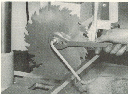
18. Place saw blade between collars. Tighten arbor nut using both wrenches.
