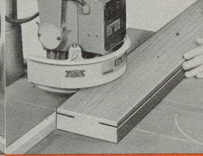
GROOVING. With material flat on the table and fed against fence, you have complete control over your work—and the result is perfect grooving!
